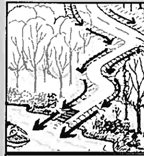
Improperly constructed and/or maintained shore-side roads can result in sedimentation to lakes and ponds.
